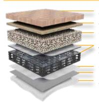
Block paving surface finish Sand bedding layer
