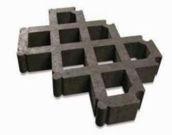
**Abweb TRP** is a no-dig or a reduced-dig, geocellular tree root protection alternative to traditional methods of constructing paths, roads and parking areas in and around trees. It is designed to protect the root structure of the tree from damage caused by the compaction of local soils as a result of vehicular traffic.
