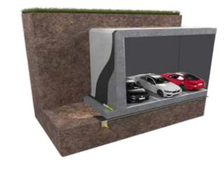
waterproofed decks, the high CBR puncture resistance protects the waterproofing from backfilling forces and root penetration, thus extending the performance and life of the system.
