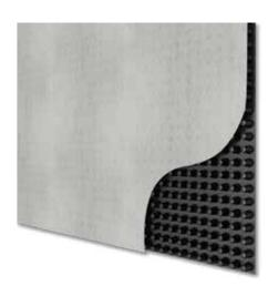
Roofdrain 60 geocomposite offers a high compressive strength and enables a shallower drainage design for podium deck structures. Using a structural geocomposite drainage core in this application means the installation time and amount of drainage stone required can be significantly reduced.
