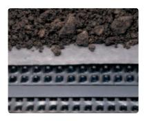
forms a high-performance free draining void, using the spacing between the cuspates. This unique core design offers clear passageways which allows flow in all directions, even in the event of damage or a blockage occurring.
