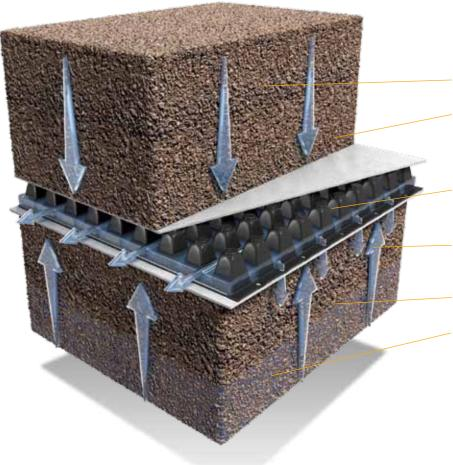
If the soil permeability is 1 x  $10^{-6}$  m/s this equates to a water volume of 1 x  $10^{-3}$  l/m²·s
