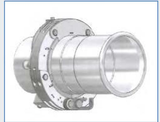
9. Perform pressing operation 1, release the catch and remove the collar. Inspect the finished joint. There will be visible witness marks from your press slings.
