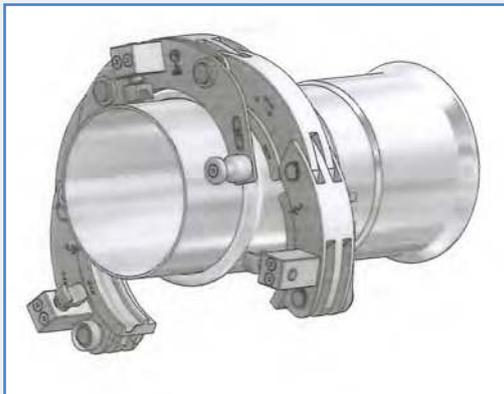
6. Open the collar and place it on the bead of the fitting (the collar joints are spring pre-loaded). Make sure that the wheels are positioned on the tube side of the fitting.
