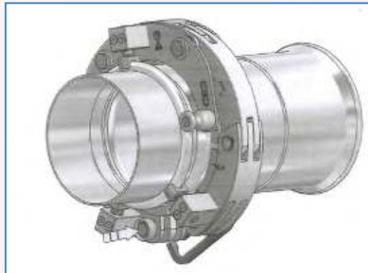
**11.** Close the collar, press the lock button, swivel the catch inwards and secure the lock.
