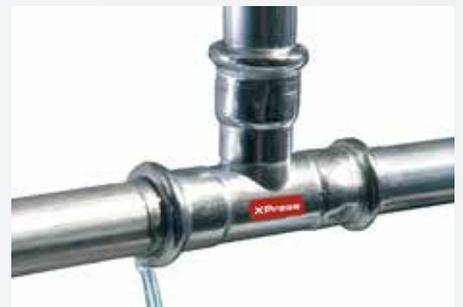
The LBP function is achieved either by a special 'O' ring or by the specific design of the fitting. This LBP function ensures that fittings, which have not been pressed, will leak during the initial pressure test. The installer can immediately see which fitting he forgot to press and correct this. Once pressed, the system is guaranteed water and air tight.
