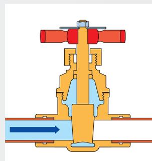
In Yorkshire gate valves the primary sealing surfaces are in gunmetal. Flow is controlled by screwing the gate into the valve body.
