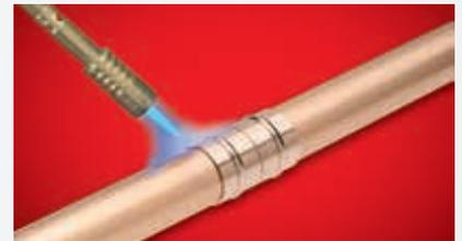
**3.** Allow the joint to cool without disturbance. Clean the joint generally, wiping off any external flux residues. This will prevent unsightly stains or (in extreme cases) corrosion of pipework. Flush out the pipework.
