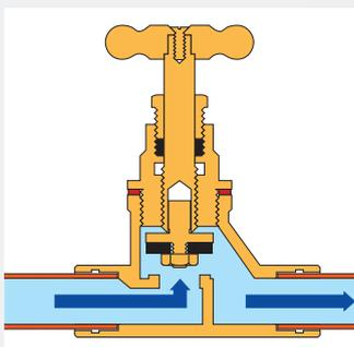
The stopvalve design incorporates a rubber washer that is screwed down onto a gunmetal seat to provide a seal against mains pressure water.
