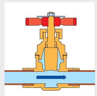
When the valve is fully open the gate moves up into the headwork to leave the flow unhindered.
