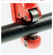
After measuring, the pipes can be cut to length using a pipe cutter, a fine-toothed handsaw or an electrical mechanical saw suitable for the pipe material. The pipe must always be cut completely through. Never partially cut the pipe and break it off as this could cause leakage. When cutting already
