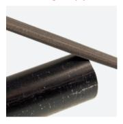
Pipe ends must be carefully and thoroughly deburred inand outside after being cut to length in order to avoid damage to the O-ring when inserting the pipe into the press fitting. A file or hand deburrer or an electrical pipe deburrer suitable for the material may be used to deburr both inside
