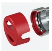
Before assembly, the protective cap has to be taken from the fitting after which the fitting must be checked to ensure that the O-rings are present and correctly positioned. Pipe, fitting and O-ring must be examined for any foreign materials (e.g. dirt, burrs), which must be removed, if present. Please
