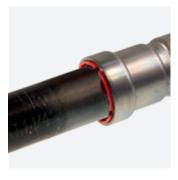
Insert the pipe carefully into the press fitting up to the marked insertion depth, without tilting, pushing it in the direction of the axis.
