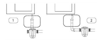
1 and 2: compulsory air intake (at inlet)
