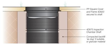
Figure 9: Installation detail A15 – areas subject to occasional vehicle loading up to
