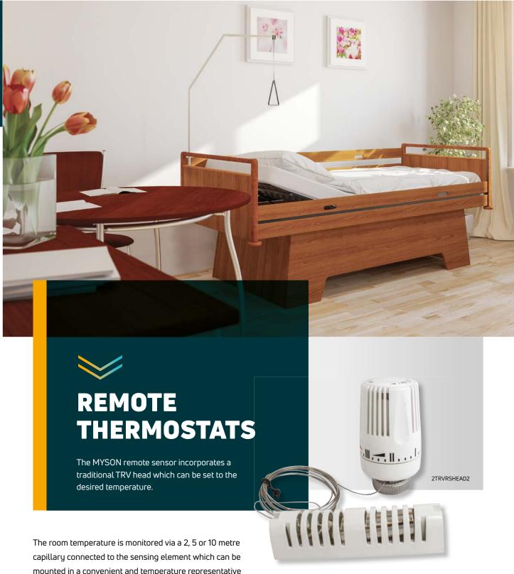
The room temperature is monitored via a 2, 5 or 10 metre capillary connected to the sensing element which can be mounted in a convenient and temperature representative area of the room. Remote sensor heads are ideal for use when it is difficult for a traditional TRV to operate, such as behind furniture or in direct sunlight, and are primarily used with LST radiators.
