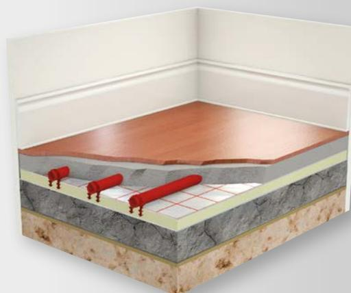
It is supplied with 25 or 50mm insulation with a webbing foil bonded to the surface. This foil acts as a protective layer, but also helps to assist the positioning of the pipework with a handy 50mm grid marked on. The pipe is then positioned in place using our exclusive Tackernails and Tackertool. It is also very flexible allowing both spiral and serpentine laying patterns.
