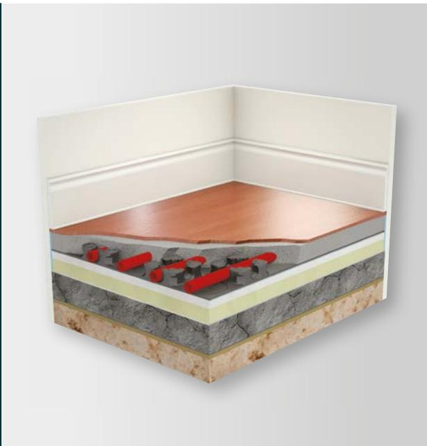
It is a castellated fixing system that comprises of an expanded 11mm polystyrene insulation base with raised burls that are designed to firmly grip the MYSON FLOORTEC underfloor heating pipe. The pipe is fixed easily into the desired pattern by lightly pressing with your foot.
