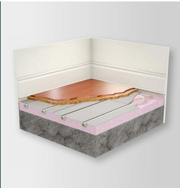
Floating floor systems have a low thermal mass and consequently have a swift response time to changes in temperature. Floating floors also reduce the overall load on the building, minimising the weight of the floor compared to the other floor systems. It is suitable for 16mm multi-layer pipework only.
