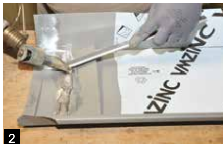
2 Solder welted strip onto panel 150mm below the water check.
