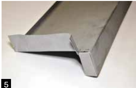
2 A hem for a single welt is formed along with a 90° return for the sill.
