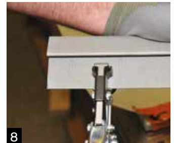
8 The strip is notched to create a friction grip.
