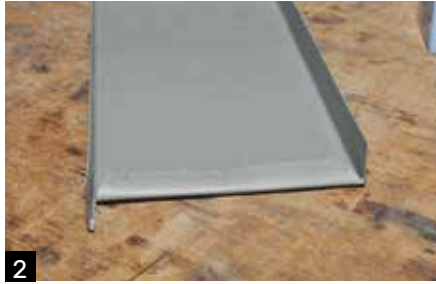
2 Fabricate the soffit panel with a 25mm hem and 2 x 25mm return folds.
