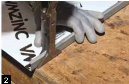
2 Straighten the upstand.
