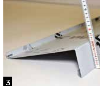
3 The sill is made with a downstand of at least 60mm.
