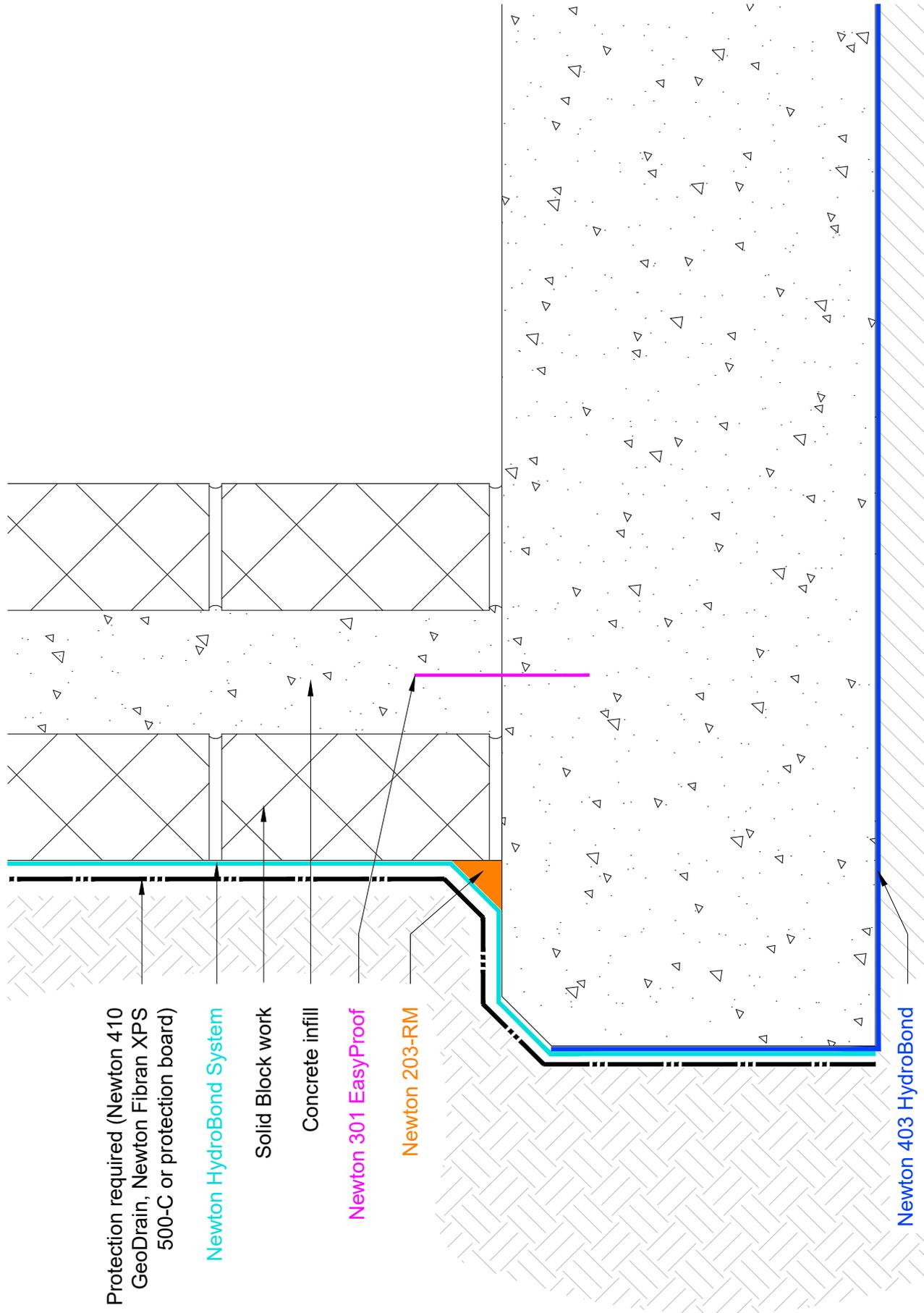
Protection required (Newton 410 GeoDrain, Newton Fibrin XPS 500-C or protection board)
