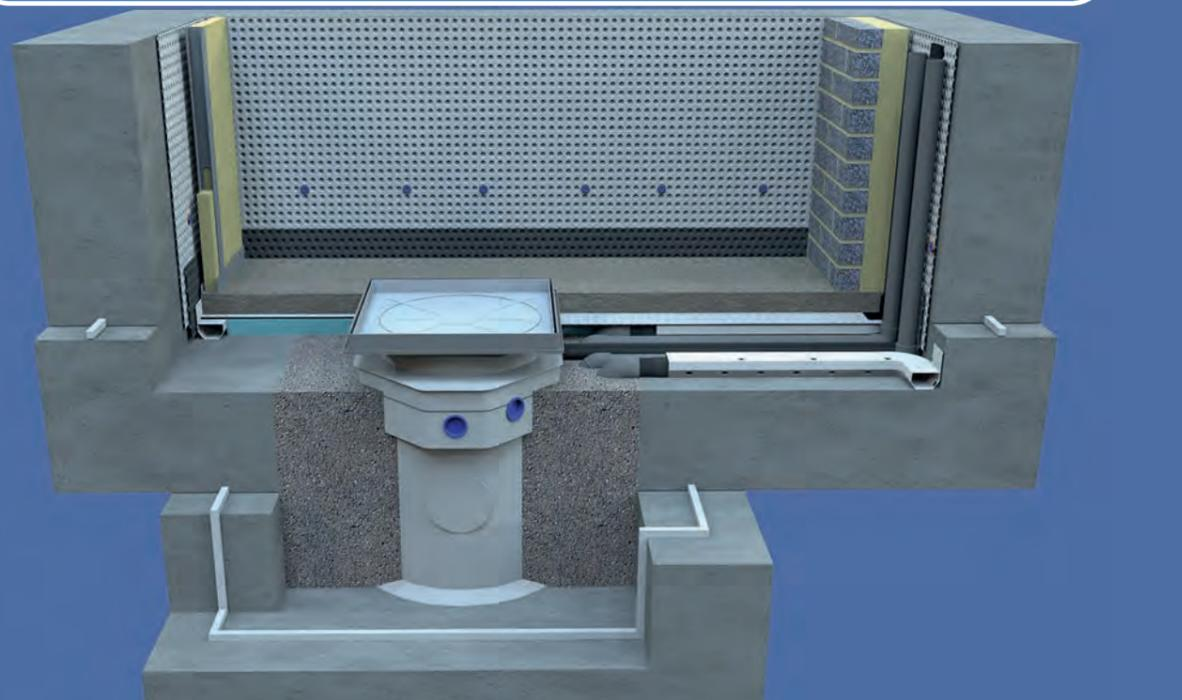
Newton cavity drain membranes are applied to the walls and floors, whilst Newton Basedrain channels collect water and provide drainage around the perimeter and above construction joints. Where removal by gravity is not possible, the Basedrain is connected to the Newton Titan-Pro pumping system to remove the water.
