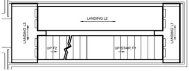
TYPE 5: Straight Flight with Intermediate Landing
