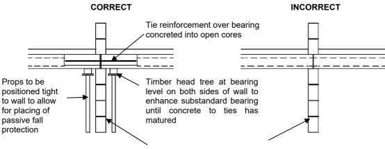
Load bearing walls less than 190mm wide
