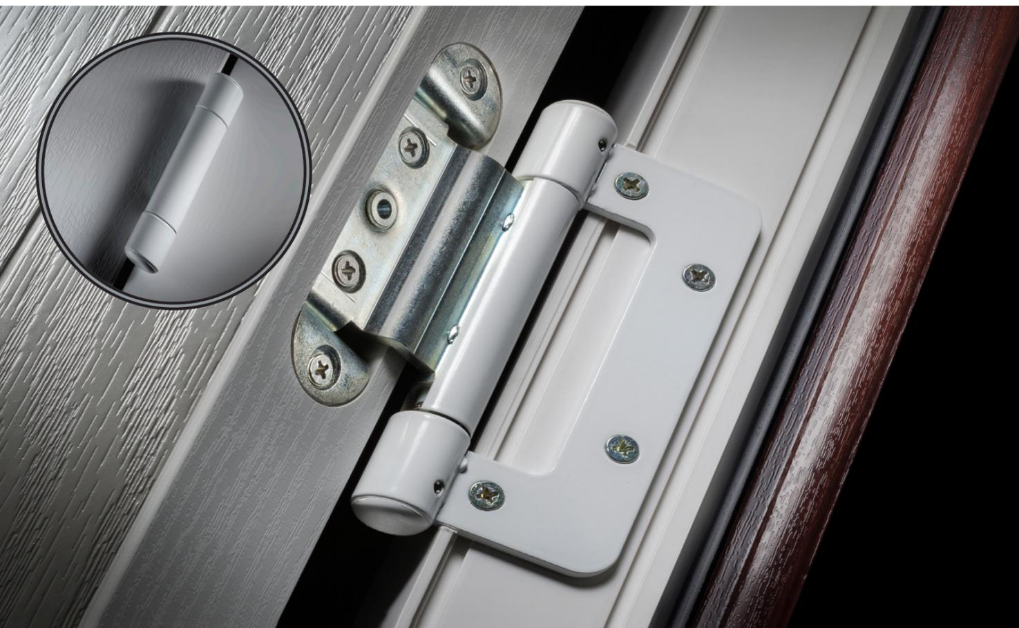
With PVC-U, composite and timber doors all being catered for, the next addition to the family was to develop a hinge specifically for the aluminium sector. Dynamic 2D-A brings the same features and benefits as all of its siblings plus a unique sash plate clamp system capable of a load capacity of 40kg per hinge. Available in mill finish, this enables systems companies to match the hinge colour exactly to the door section for each project.
