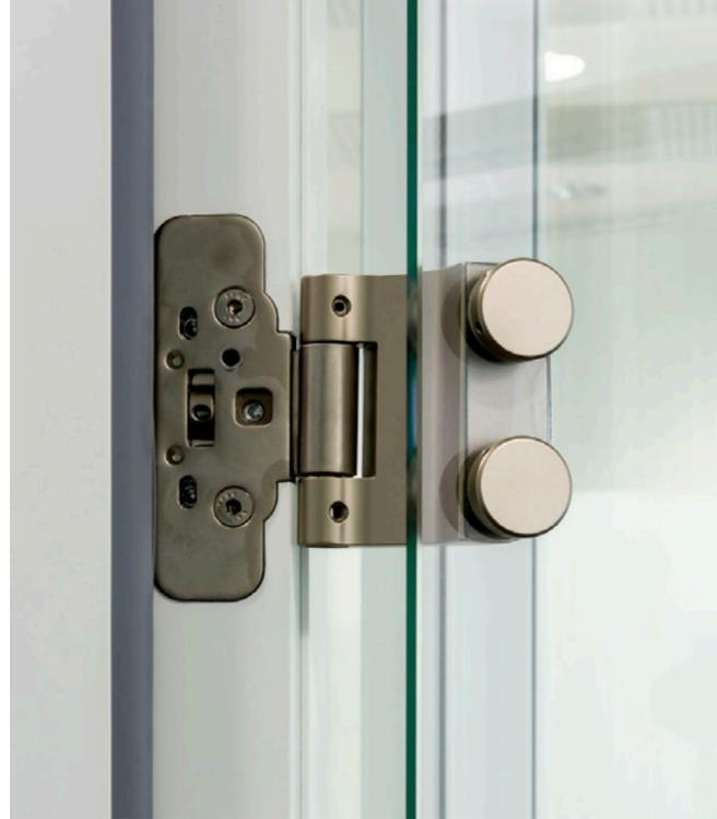
Just 3D for glass doors increases the range of this product. By keeping all the adjustment characteristics in the three dimensions of the other applications, this hinge has been designed to be applied on flush door frames from 40 to 44 mm.
