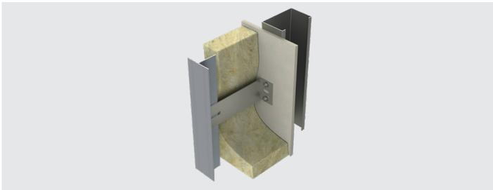
For greater performance SFS have recently introduced a complete range of stainless steel brackets to complement our vertical aluminium ranges. Our stainless steel range is made from superior 316 grade which exhibits far greater resistance to localised corrosion in marine and in contact with atmospheric pollution found in most built up environments.
