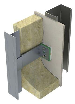
Whilst strong and easy to install aluminium is very thermally conductive e.g > 200 W/mk. Therefore the thermal point loss affects can be significant when aluminium brackets are utilised depending on the combination of various elements within the rainscreen build-up.
