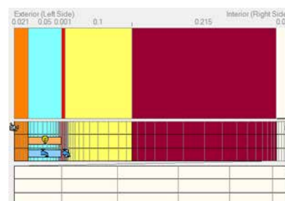
Rainscreen Brick Wall with external PIR/Rockwool
