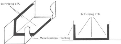
Fireplug ETC Electrical Trunking Closers are made to suit the various sizes of trunking. Two Fireplug ETC are supplied up to 3" x 3". Three Fireplug ETC are supplied for larger sizes.
