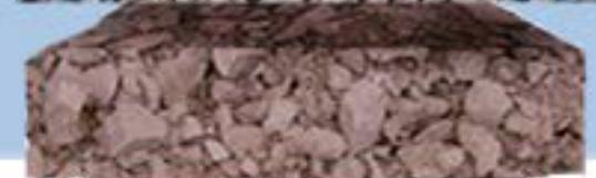
A 150mm - 225mm layer of Type 3 granular sub-base
