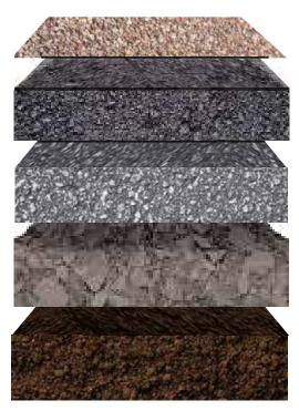
**Addastone PLUS Resin Bonded -** Typical depth 5-7mm depending on aggregate size
