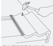
Fig. 4 - Mechanically fix verge unit
