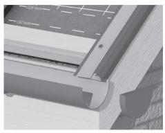
Fig. 19 – Nail each length of trim to batten
