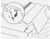
Fig. 3 - Allow play for verge unit to slide down
