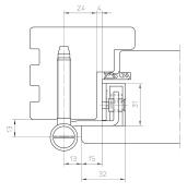
e.g. BAKA Protect 2010 2D 15 mm overlap without overlap seal
