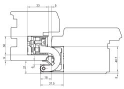
for overlap widths from 21 - 27 mm e.g. overlap width 21 mm
