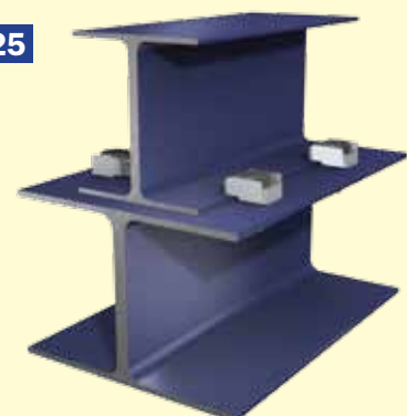
Drilled I-Section running parallel to another I-Section
