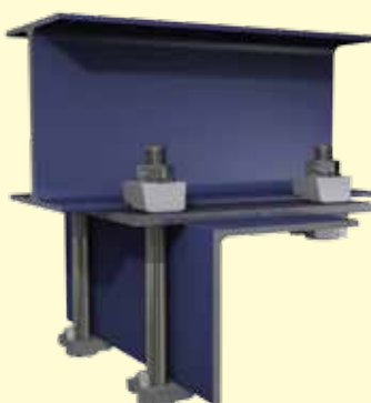
Angle section below an I-Section at 90 degrees
