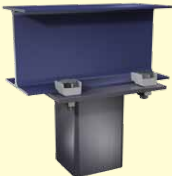
Column end plate to I-Section
