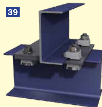
Channel positioned above I-Section at 90 degrees
