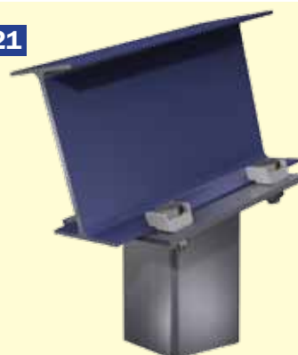
Column end plate to sloping I-Section
