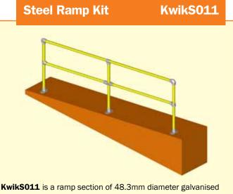
**KwikS011** is a ramp section of 48.3mm diameter galvanised steel handrailing 3000mm long with three uprights and angled flat fix baseplates. The handrail accommodates variable ramp inclines from 0–11 degrees.
