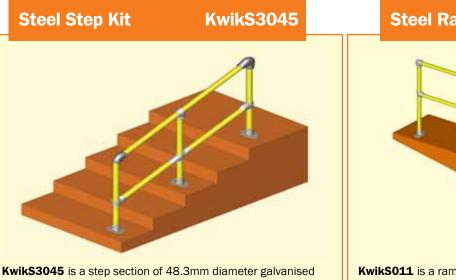
**KwikS3045** is a step section of 48.3mm diameter galvanised steel handrailing 3000mm long with three uprights and flat fix baseplates. The handrail accommodates variable step inclines from 30–45 degrees.
