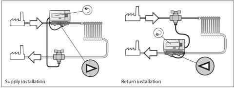
Heat meters have red temp sensor in supply pipe and all cooling meters have blue temp sensor in supply pipe
