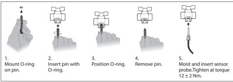
To ensure accuracy and a tight seal the sensor installation should comply to EN1434-2 annex A:
