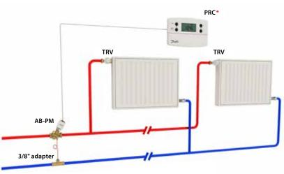
AB-PM: Pressure differential controller with flow
