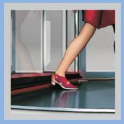
A Heel Sensor is fitted to the bottom rail of each door leaf. The door will stop rotating when the buffer is compressed and when the obstacle is removed the door will begin rotation as normal.
