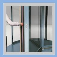
A 30mm Passive rubber buffer safety device is fitted to both entry sides of the drum wall and a 30mm Horse Hair brush strip is mounted within the nose of the door to seal the door leaf against the drum wall. The door will stop rotating when the buffer is compressed and when the obstacle is removed the door will begin rotation as normal.
