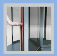
A 30mm rubber buffer is fitted to both entry sides of the drum wall and a 30mm Horse Hair brush strip is mounted within the nose of the door to seal the door leaf against the drum wall. This prevents hands and fingers being trapped between the door leaf and drum, whilst keeping a constant seal on the door.
