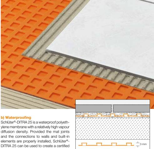
Schlüter®-DITRA 25 is a waterproof polyethylene membrane with a relatively high vapour diffusion density. Provided the mat joints and the connections to walls and built-in elements are properly installed, Schlüter®-DITRA 25 can be used to create a certified bonded waterproofing assembly with the tile covering. Schlüter®-DITRA 25 features the national technical approval (abP) required in Germany and bears the Ü mark. Moisture exposure class according to abP: 0 - B0 as well as A and C.
