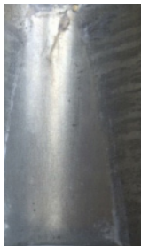
After 6 weeks salt spray test
