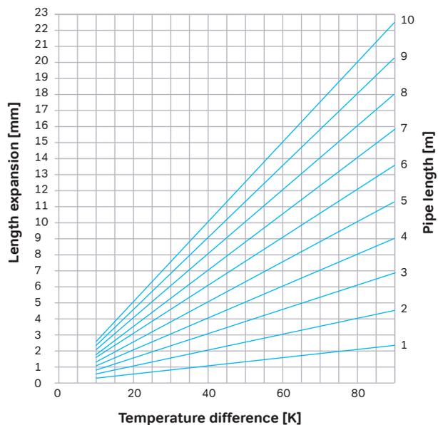
Figure 31: Calculation example length change.
