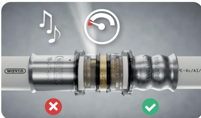
With ACOUSTIC LEAK ALERT any un-pressed fitting emits a loud whistle ( $\pm 80 \text{ dB(A)}$ )<sup>3)</sup>, making locating the source of the leak extremely easy. And, because unpressed fittings are detected so quickly, Tigris M5 and Tigris K5 fittings make testing with air an unbelievably attractive alternative.
