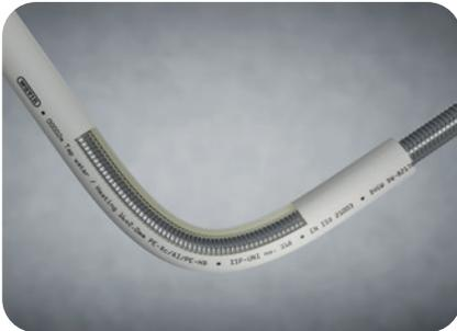
By bending the pipe the demand of fittings needed for the installation can be reduced. The pipe is easy to bend: by hand, with the aid of the bending spring or using the Wavin bending pliers. Bending springs and bending pliers are preferred to be used to ensure the pipe is not kinked by accident. Larger diameters can be bent with pliers with appropriate dimensions, bending radius min. 3xDa.
