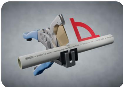
Figure 19: Calibrating the pipe.
