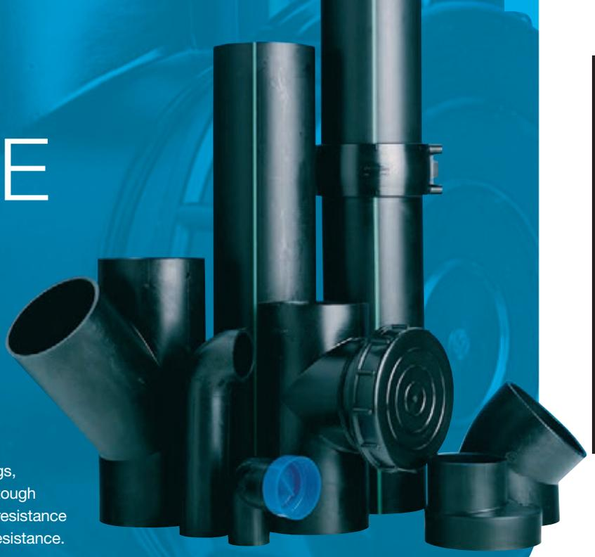
Wavin HDPE pipes and fittings are jointed by welding, making the joints resistant to tension. There are two methods of welding: butt welding and electro-fusion welding. Most Wavin HDPE products can also be used as part of negative pressure installations like the siphonic roof drainage system Wavin QuickStream.
