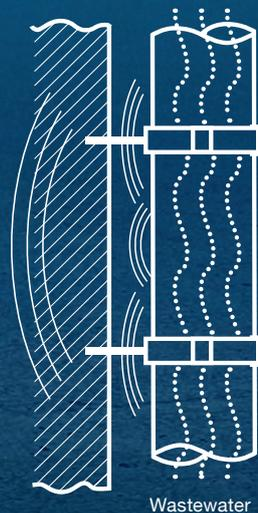
**Structure-borne** sound is the amount of noise that can be heard from the pipe after the noise has permeated through pipe supports, brackets and walls
