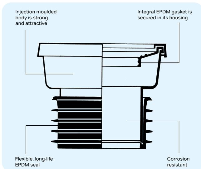
Figure 19: Connection to ground floor WC
