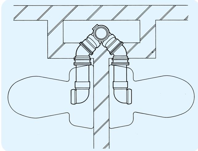
Figure 22: Alternative back-to-back WC installation
