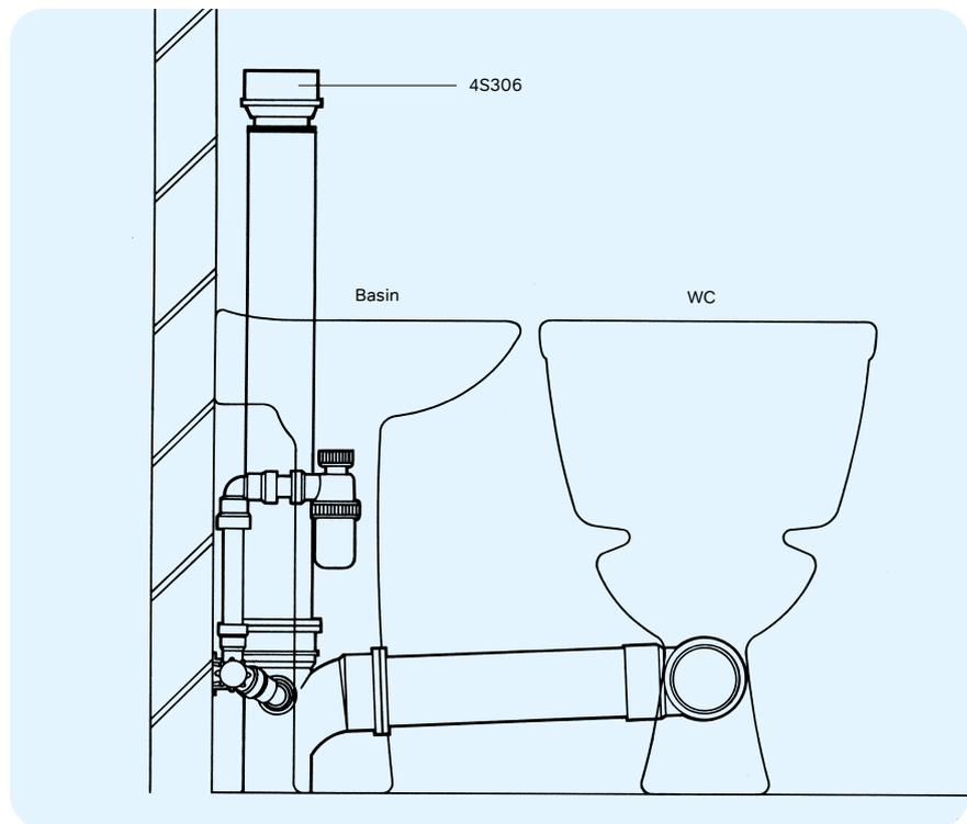
Figure 26: Examples of provisions for drain ventilation
