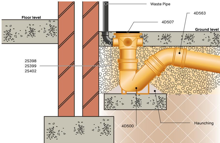
Figure 8: Typical waste pipe connection to Bottle Gully
