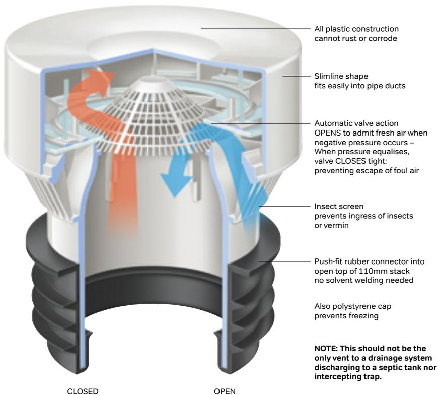
When used to vent a soil stack, 110mm Air Admittance Valve 4S306 should be located:
