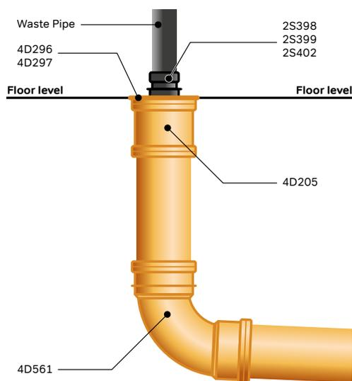
Figure 7: Typical waste connection to Sealed Hopper
