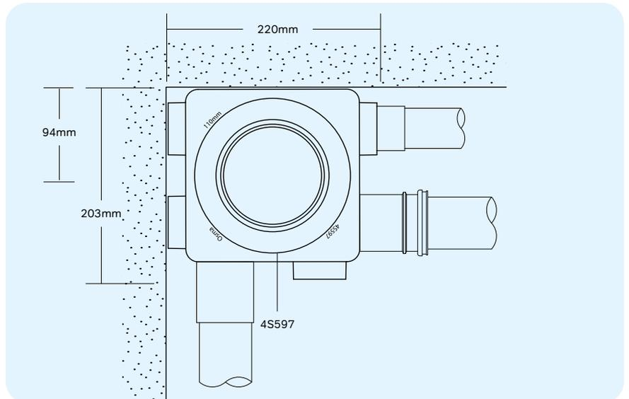
The 6 Boss Soil Manifold – 4S597 is a compact fitting designed for easier installation where space is restricted. It is particularly suitable for multi-occupancy residential buildings.
