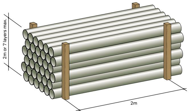
Figure 30: Storage of loose pipe on bearers
