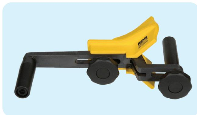
For connections to Wavin AS+ fittings or sockets the pipe end needs to be chamfered. It is recommended to chamfer over a length of 5mm under a 15 degrees angle. This can be done by using standard chamfer tooling.
