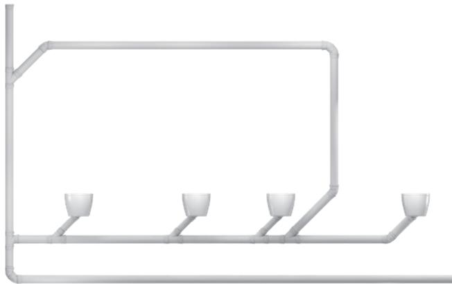
Figure 13: Air-circulation pipe.
