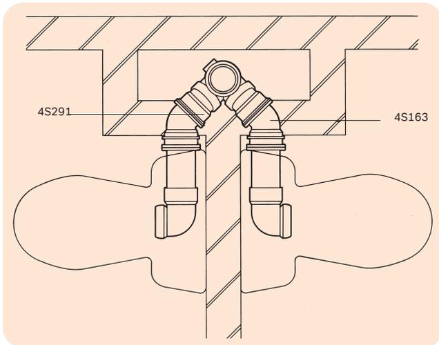
Figure 27: Alternative back-to-back WC installation
