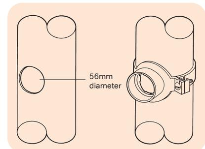
Figure 60: Fitting Boss Socket Adaptor
