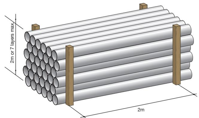
Figure 40: Storage of loose pipe on bearers
