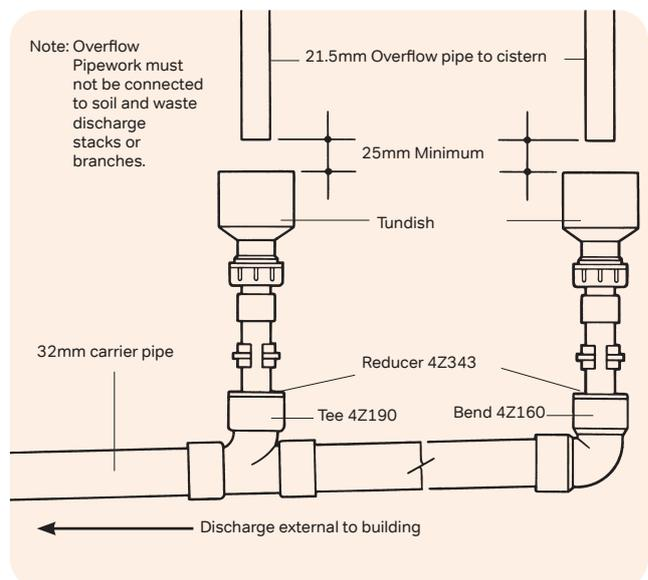
Figure 72: Tundish connection to 21.5mm Push-Fit Overflow Pipe
