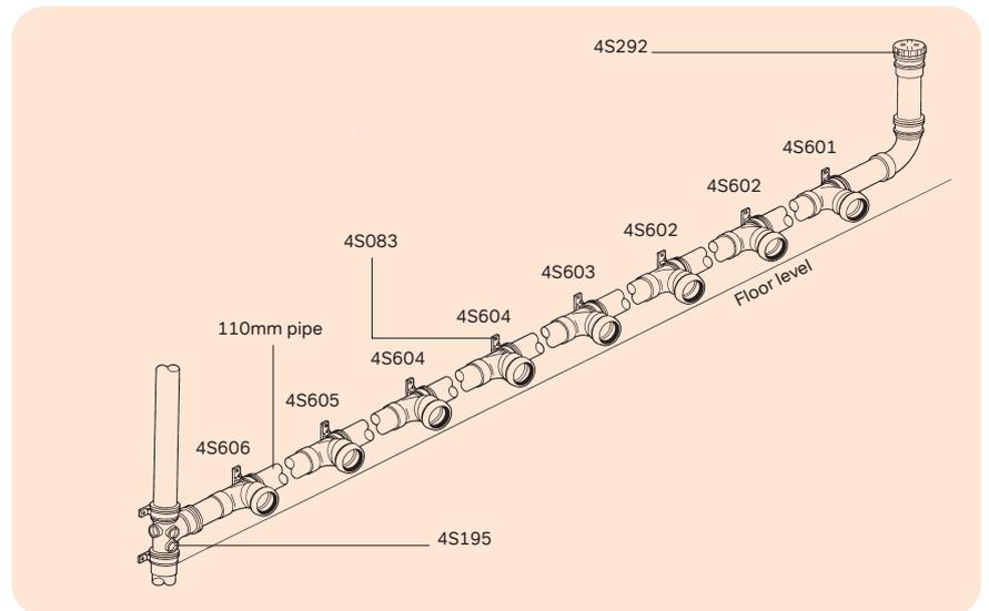
Figure 30: Typical layout of double manifold float
