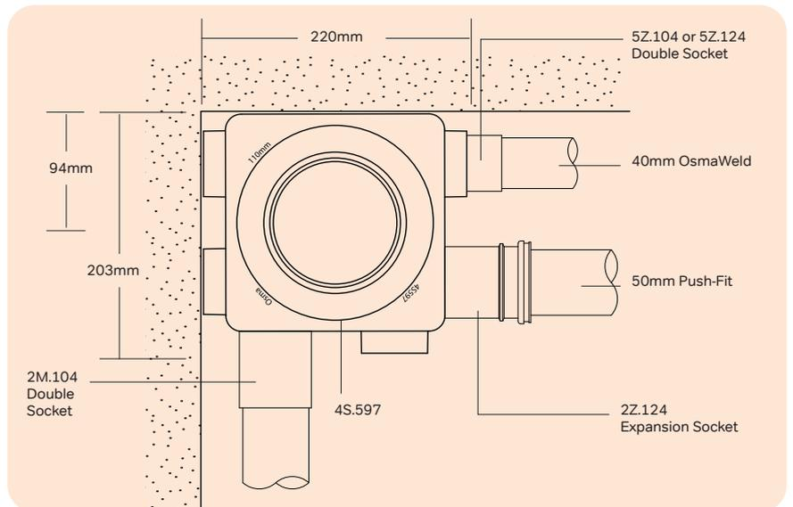
Figure 19: Typical Bathroom Installation using 6 Boss Soil Manifold 4S597
