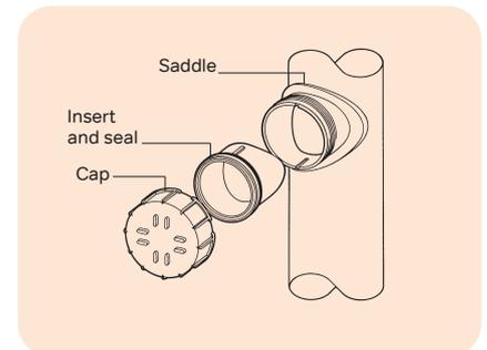
Figure 52: Installation of Access Saddle
