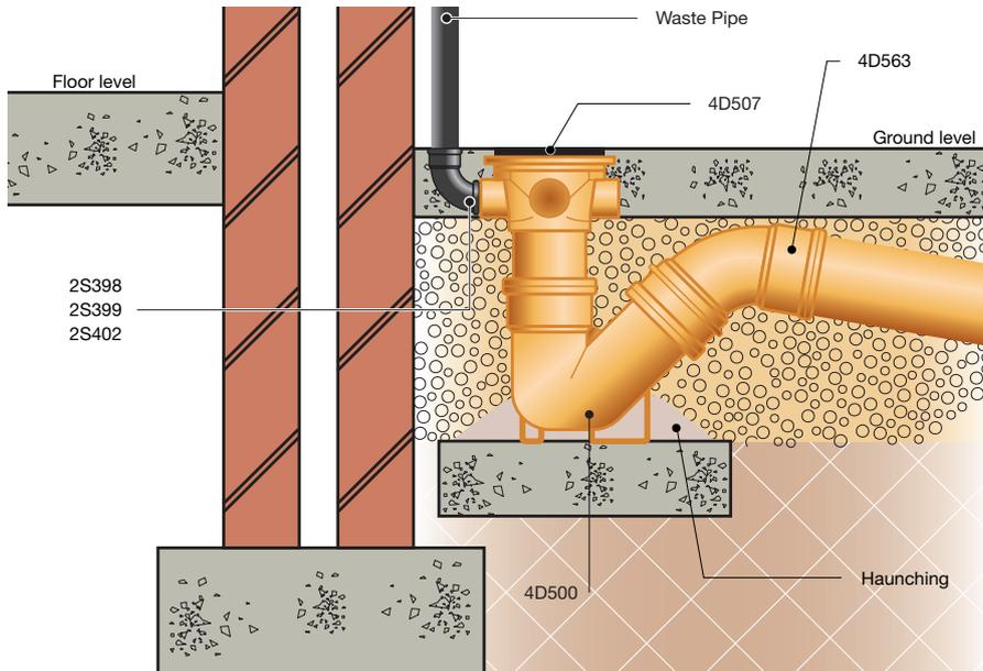
Figure 13: Typical waste pipe connection to Bottle Gully
