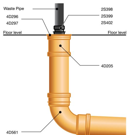
Figure 12: Typical waste connection to Sealed Hopper
