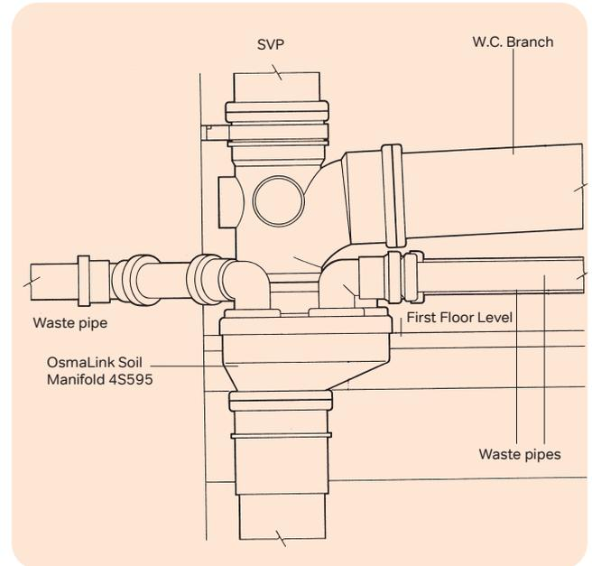
Figure 62: Typical OsmaLink Soil Manifold installation (plan view)
