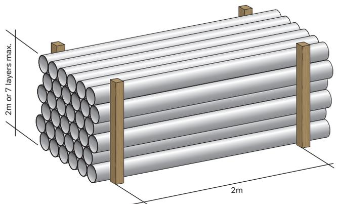
Figure 22: Storage of loose pipe on bearers
