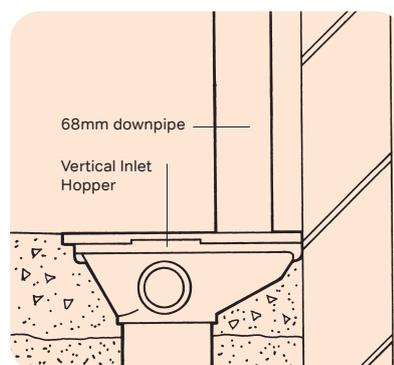
Figure 18: Connection to bottle gully
