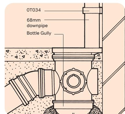
Table 10: Connections to Below Ground Drainage
