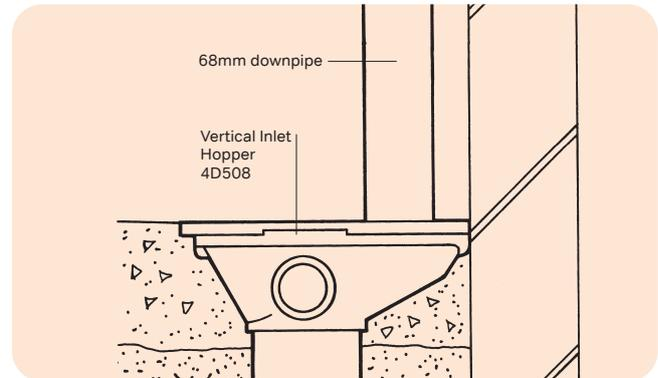
Figure 56: Connection to Bottle Gully (61mm square pipe illustrated)
