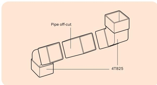
Figure 46: RoofLine shallow offset
