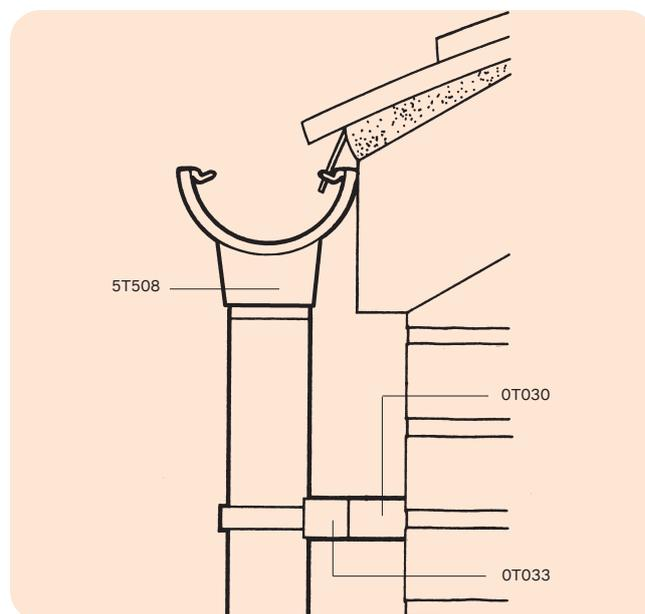
Figure 9: Use of Pipe Bracket Spacer
