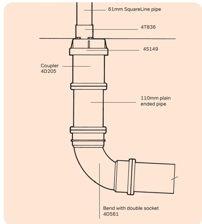
Figure 50: Connection to 110mm PVC-U Socket (61mm square pipe)
