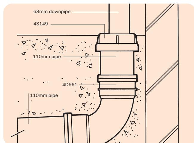
Figure 49: Connection to 110mm PVC-U Socket (61mm square pipe)
