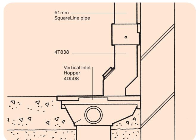
Figure 57: 110mm Connection to PVC-U Drain Socket
