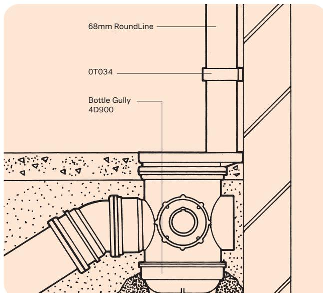
Figure 55: Connection to Bottle Gully (68mm Circular pipe illustrated)
