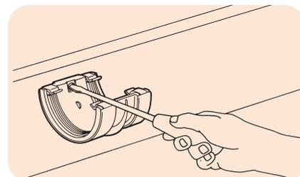
Figure 27: Installation of RoundLine Gutter Union
