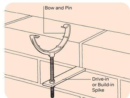
Figure 34: Installation of Rise and Fall Brackets
