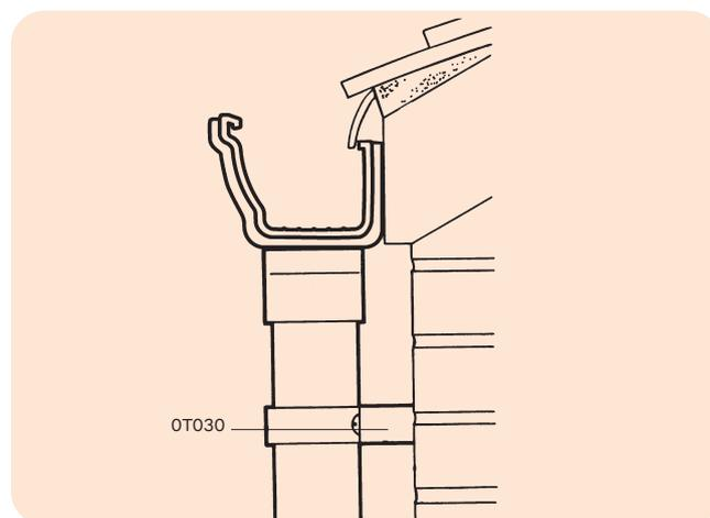
Figure 44: Application of Pipe Bracket Spacer
