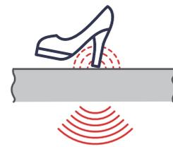
⌚ **Impact sound** is a special form of structure-borne sound caused by footsteps or falling objects. It propagates as airborne sound
