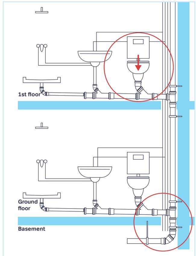
Figure 48: Main sound sources according to DIN 4109
