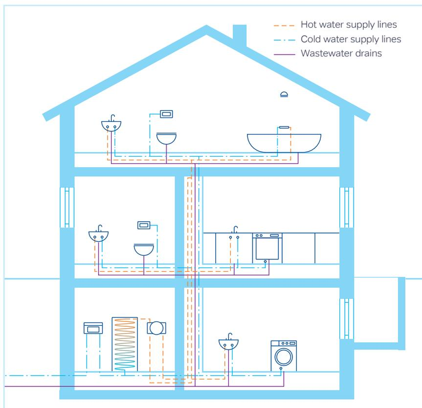
**Figure 15:** Supply and disposal lines in a building
