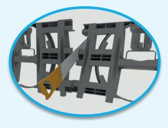
**Note 2:** After cutting there is a left and right version. Be sure that the rounded edge of the half panel is positioned towards the corner of the system (not the cut edge!) or depending on the length of the side, put the half panel in between two uncut panels.
