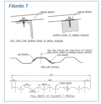
Recommended purlin and vertical rail centres 1m. Note that, although shatter resistant, Filonite is flexible and must not be stood on when on the roof. It is recommended that a sealing tape is used at side lap positions as illustrated
