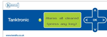
The LED will turn green, indicating normal operation; if the status LED remains red check the 'Alarms' status and rectify the problem. See FAQ's if necessary.
