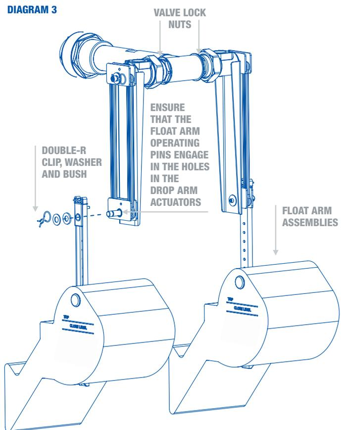
**9** If the valves are not level, each individual valve can be rotated at its screwed connection into the T-outlet. This joint is sealed by an “o”-ring so can be moved without fear of a leak.
