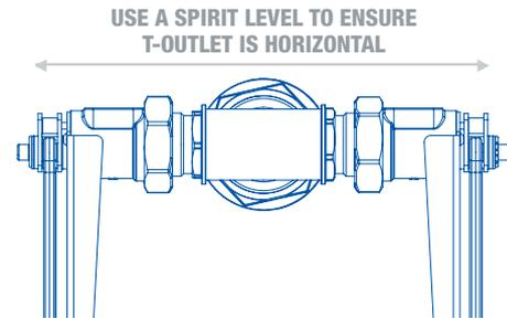
**7** Tighten the backnut sufficiently to hold the complete valve in position but note that it may be necessary to move the valve later after the float clearances have been measured.
