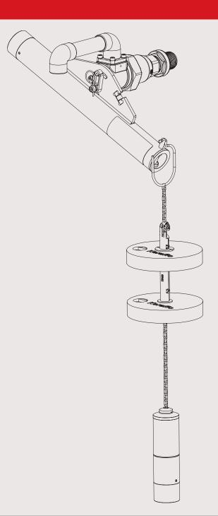
**KERAFLO** float valves contain a pair of maintenance free ceramic discs.
