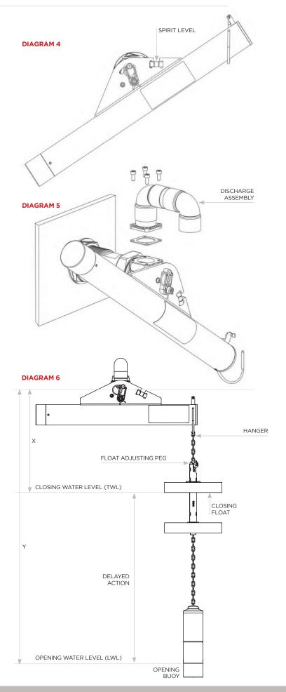
Adjust the length of the chain from the buoy to the hanger to match the following:
