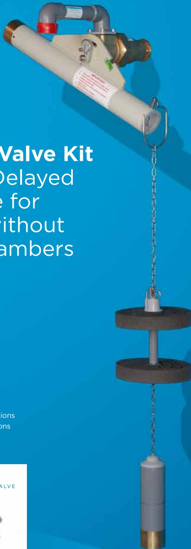
The KP Type Float Valve Kit comprises an in-line Control Valve together with an Aylesbury KB Type valve acting as a pilot. The pilot valve offers fully variable delayed action opening and closing water level settings, making this ideal for mains or pumped systems.
