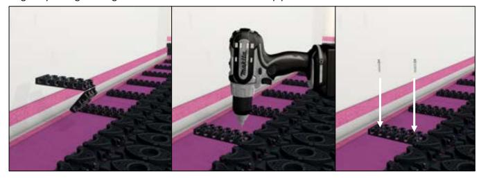
Profix® Clip-Rails can also be used in close proximity to the manifold to secure pipework at close centres prior to transitioning into the Profix® Panels themselves.
