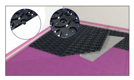
Profix<sup>®</sup> Clip-Rails supplied within the Profix<sup>®</sup> Manifold & Highway Pack can be used to create a 'highway' along the edge of a room to facilitate additional pipe runs from and back to the manifold.
