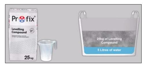
Apply Profix® Levelling Compound to minimum 15mm thickness for tiles or engineered wood flooring. Apply additional minimum 3mm Profix® Levelling Compound for carpet or vinyl flooring.\*
