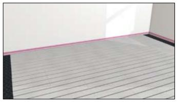
Profix® Clip-Rails can be used in close proximity to the manifold to secure pipework at close centres prior to transitioning into the Grooved Dry Screedboards.
