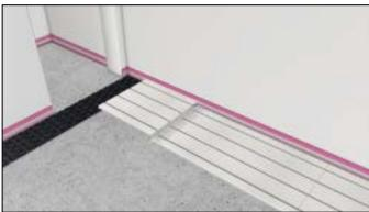
Work your way back up the room to form the second row of Grooved Dry Screedboard, ensuring that a bead of Screedboard adhesive is applied to every T & G joint, cutting to length the final board in the row as before. Follow this process one row at a time, ensuring that the boards are installed in a continuous brick-bond pattern.
