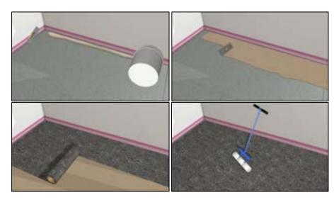
Smooth out the surface of the mats using a roller, pressing down firmly to ensure good adhesion and to remove any air bubbles. Foot traffic should be avoided for 24 hours, while the adhesive dries, before installing the Profix® Panels onto the acoustic isolation mats.
